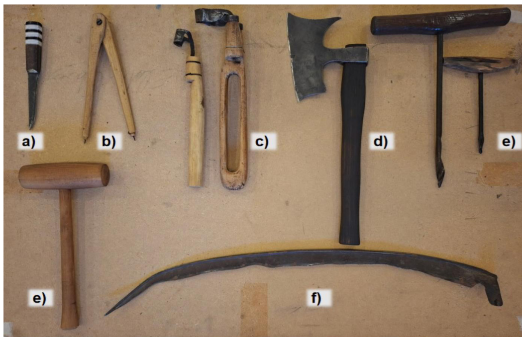
Slika 6. Alati kačarskog zanata: a) kovani nož; b) drveni šestar; c) mamlje; d) bradva/bradvin; e) svrdla/bugije; e) drveni čekić; f) kosa/diljač / Image 6. Tools of the cooperage craft: a) forged knife; b) wooden compass; c) drawshave; d) hatchet; e) drill; e) wooden mallet; f) scythe
